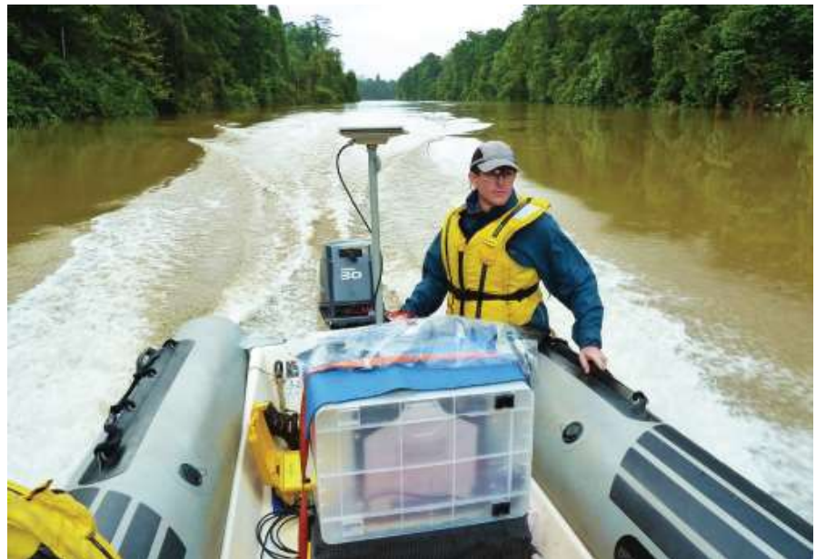
Jeremy Schierer, a YWAM volunteer and master mariner, uses the CEESCOPE Echo Sounder to chart a river in Papua New Guinea. (Photo courtesy of YWAM)
