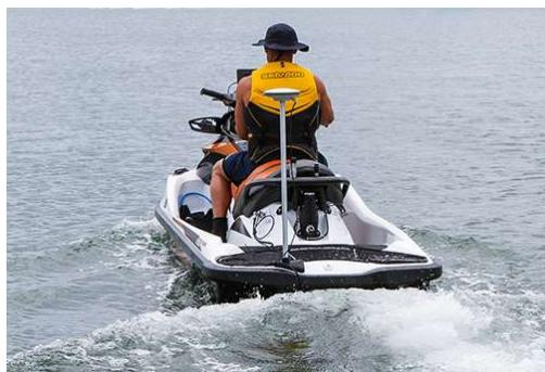
With a survey-grade CEESCOPE™ single beam echo sounder, RTK GNSS, on-board computer for data collection, and HYPACK® software, the CEE JET™ allows collection of high quality bathymetry data in the often substantial area of the surf zone. The CEE JET™ is a standard Sea-Doo personal watercraft (PWC), modified at the CEE
