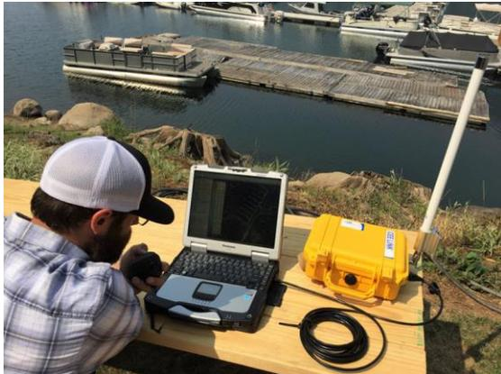
The dedicated CEE LINK™ base station includes a high-power radio to receive data even if the vehicle is located behind obstructions, in this case moored boats. Real time review of sounding quality happens throughout data acquisition, in this case using Eye4Software Hydromagic.
