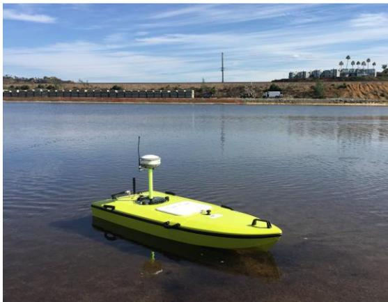
The lagoon environment has no tidal exchange and soft mud banks presented an impossible task for a manned boat survey and so a USV was the obvious solution. Local control was provided for the survey using a Hemisphere S320 GNSS base station with UHF radio, transmitting corrections to Coastal's own S320 RTK rover installed on the USV. GNSS data were incorporated into the USV's CEESCOPE-LITE™ control system using a Bluetooth link from the S320 rover
