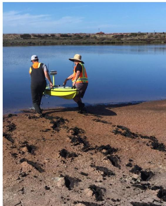
After launching the CEE-USV™, a perimeter was established by walking with the boat around the lagoon. Thereafter, a set of repeatable planned lines were followed within the perimeter boundary. Having more power than necessary for this small survey was useful as the USV was able to simply drive right through the soft surface sediment instead of getting stranded.
