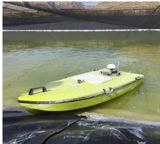
The boat was first driven around the perimeter of each pond, and then with the edge of the survey established it was driven in a standard line pattern from two, or in the case of the longest 500m (1600ft) pond, three control positions on the shore. With winds at 25-35mph, the low windage of the USV helped the vessel stay on track although frequent course correction was still required to keep on line.
