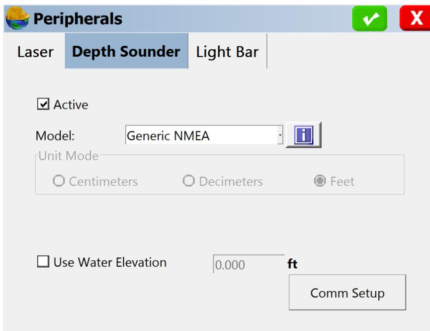
The Comm Setup should match the serial port of the Carlson device. The baud rate is 9600, Parity is None, Data Bits is 8 and Stop Bits is 1. Port 5 shown below is only for this demonstration.
