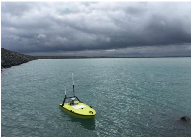
CEE-USV™ with autopilot and long-range antennae.
