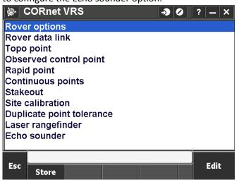
Select Echo sounder > Edit and set type as DBT (options are CEESTAR HF, CEESTAR LF, NMEA SBDBT, Sonarmite). The controller port is set to Bluetooth. Latency is typically 0.0s. Enter draft to reference transducer face to GNSS offset reference level.
