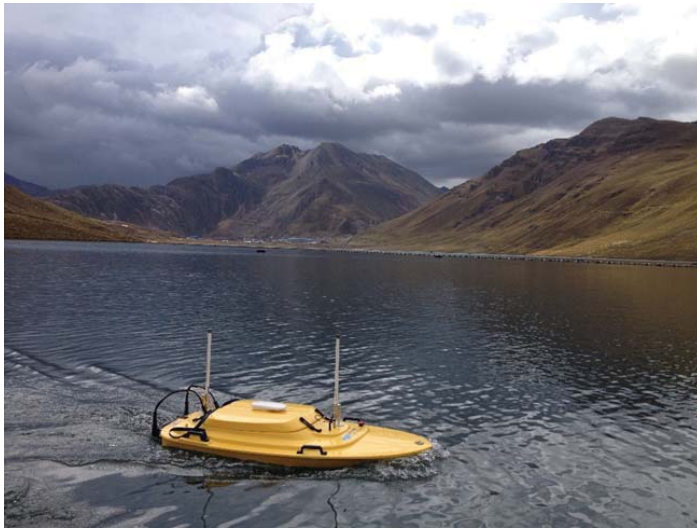
Figure 3. Unmanned surface vehicle (USV) collecting data in Perú at an elevation above 4000 m.
