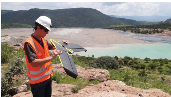
Figure 1. Inspecting an unmanned aircraft system (UAS) prior to launch.
