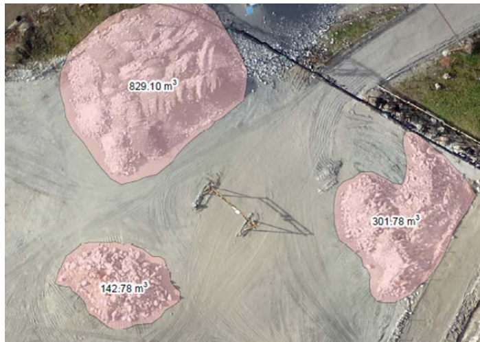
Figure 5. Example of stockpile volume estimation in Perú using UAS software and aerial imagery
