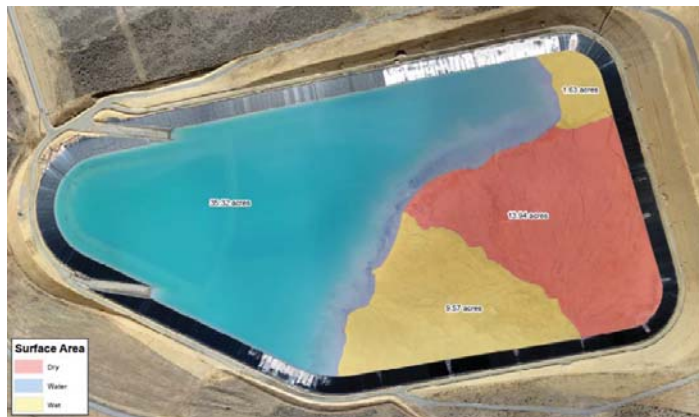
Figure 6. Surface moisture mapping using UAS data, northeastern Nevada.
