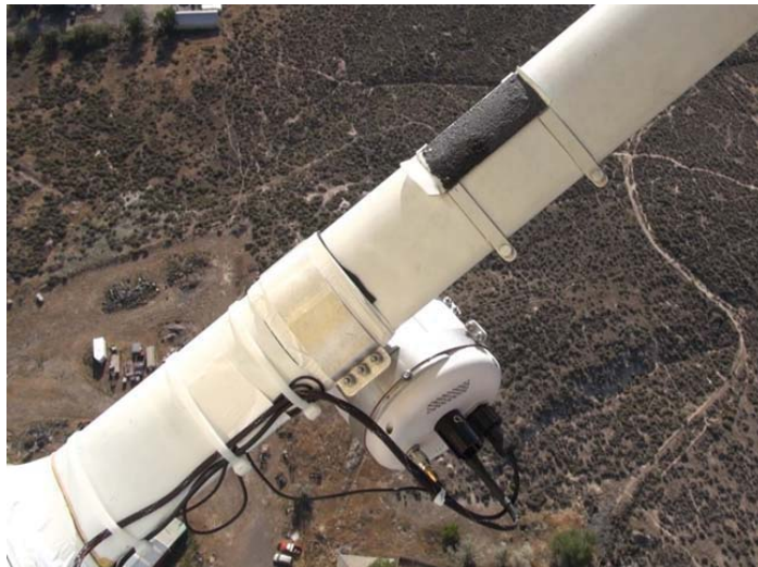
Figure 2. Manned aircraft system (MAS) mounted on a fixed-wing aircraft.
