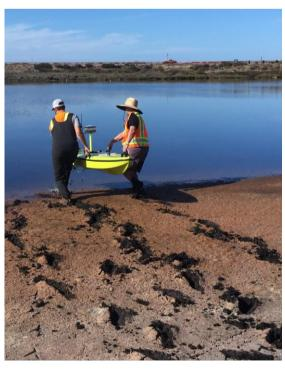
After launching the CEE-USV™, a perimeter was established by walking with the boat around the lagoon. Thereafter, a set of repeatable planned lines were followed within the perimeter boundary. Having more power than necessary for this small survey was useful as the USV was able to simply drive right through the soft surface sediment instead of getting stranded.
