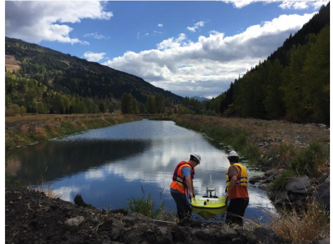
Figure 6. Deploying the CEE-USV in a coal mine pond.
