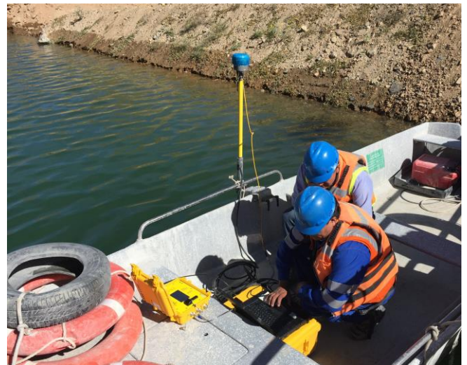
Figure 4. Interfacing site RTK and CEE ECHO™ sonar.
