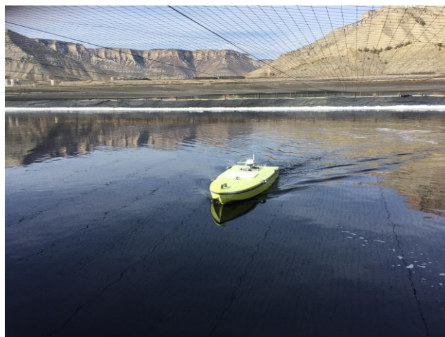
Figure 11. USV under netting in baking soda plant.
