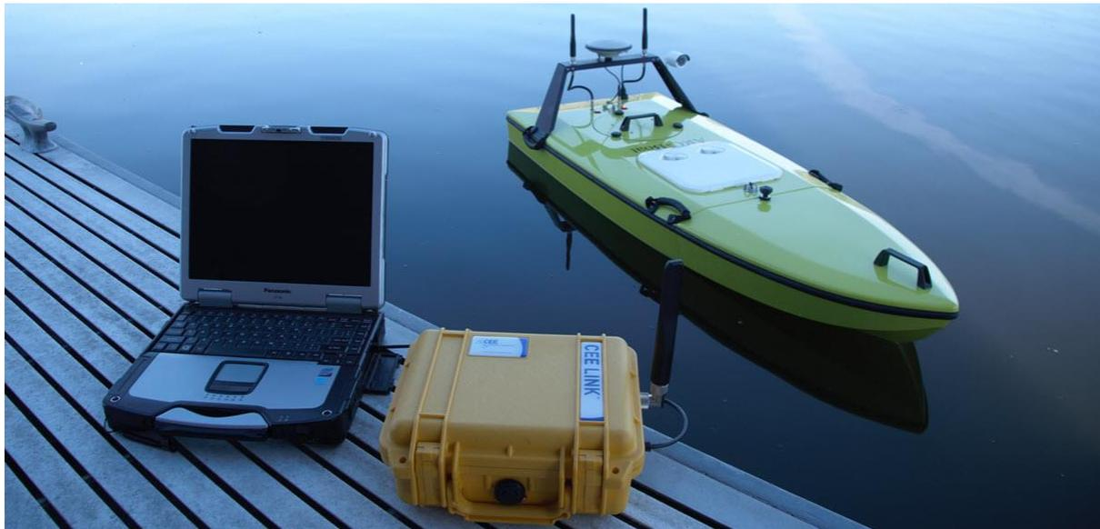
**Simplicity of Operation.** A survey tool not a science project; simply turn on the vehicle and the on-board CEESCOPE™ and start surveying. With echo sounding, positioning, data management, user control interface, RTK and data telemetry in a single enclosure there is no simpler USV to use. Minimize downtime, mobilization, and field crew headaches.
