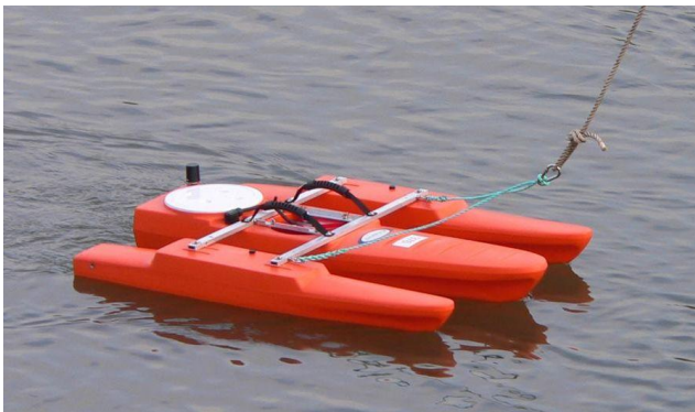
Tethered float and ADCP used for previous surveys.
