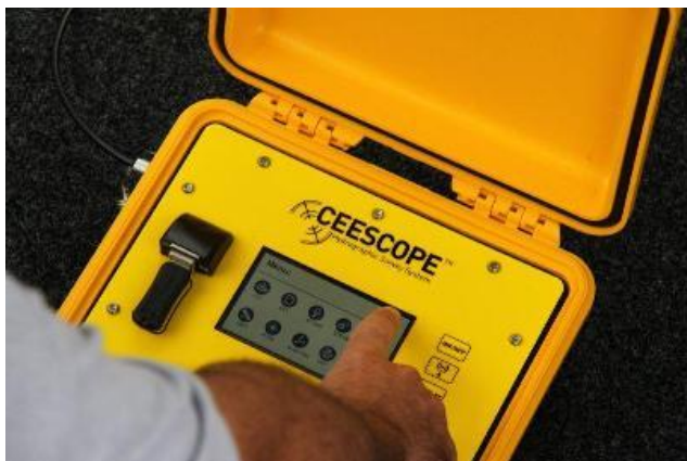
CEESCOPE™ "all in one" GNSS and echo sounder.
